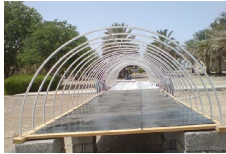
(a) Tunnel placed on concrete block substructures showing collector part (black painted metallic sheets)
